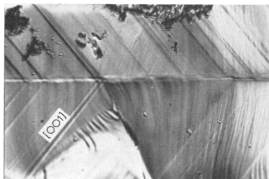
Figure 3 An interference contrast micrograph of a (010) face across a twin boundary illustrating the deviation of [001] slip steps across the boundary ( \times 225 ).
